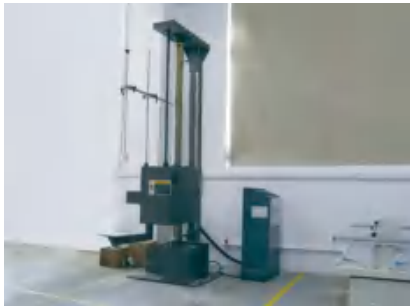
Arm drop test machine
