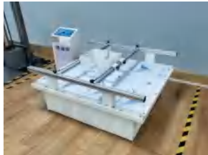
Transportation vibration testing
