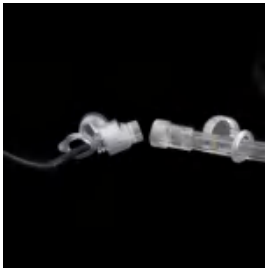
Power cable connector to Strip
