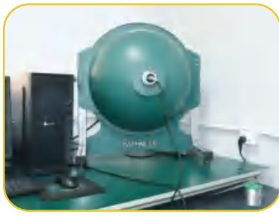
LED Testing before SMT
