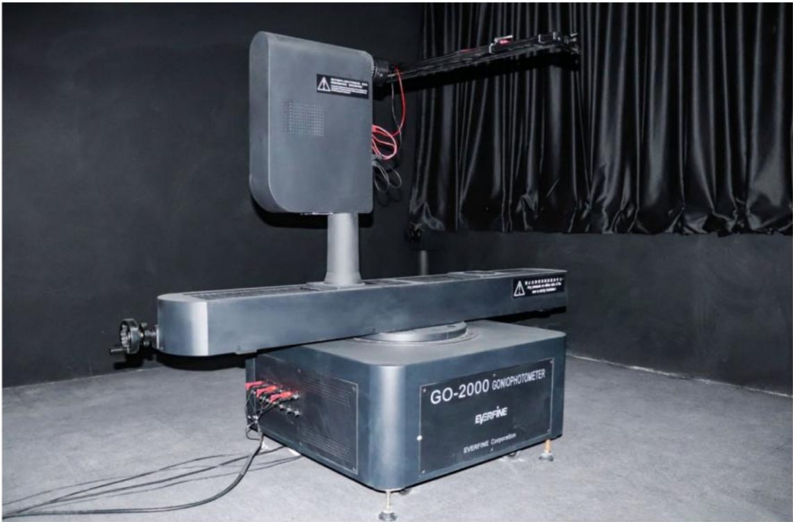
GO-2000 Goniophotometer Testing Lab
