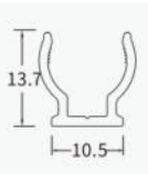
PC clips 20x10.5x13.7mm(L x W x H) Accessories:Screw M3x15mm
