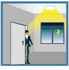
When motion is detected, the sensor brightens the lamp to 100% illumination.
