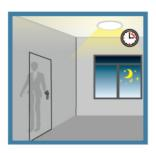
After the hold time, the sensor dims the lamp at the preset low light level if no motion is detected.
