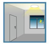
No motion detected, the lamp remains at a low light level all the time.
